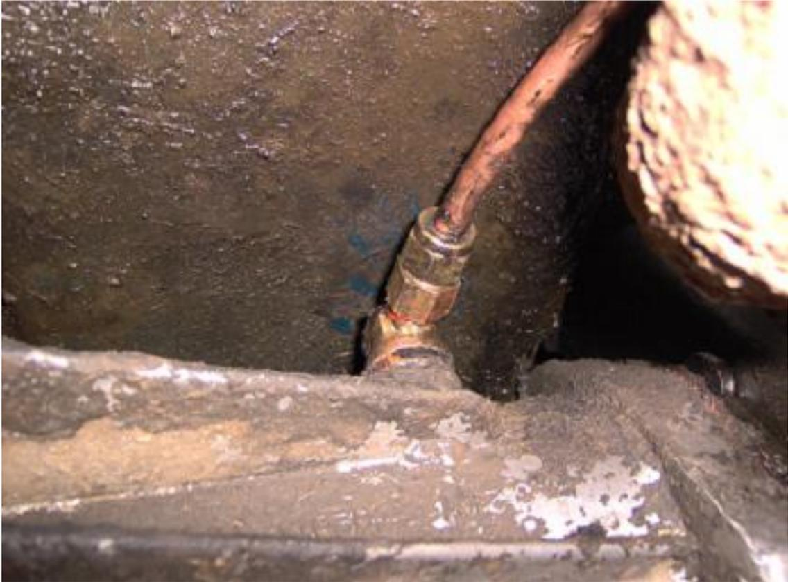
I smeared a little red RTV on the breather lower part before installing it back in the diff case. Now is time to do a series of bends on the copper tubing in order to clear both the exhaust manifold and main steering rod. The PVC hose is then fitted to the free end of the tubing and routed to the hose manifold (keep on reading for more on this).
