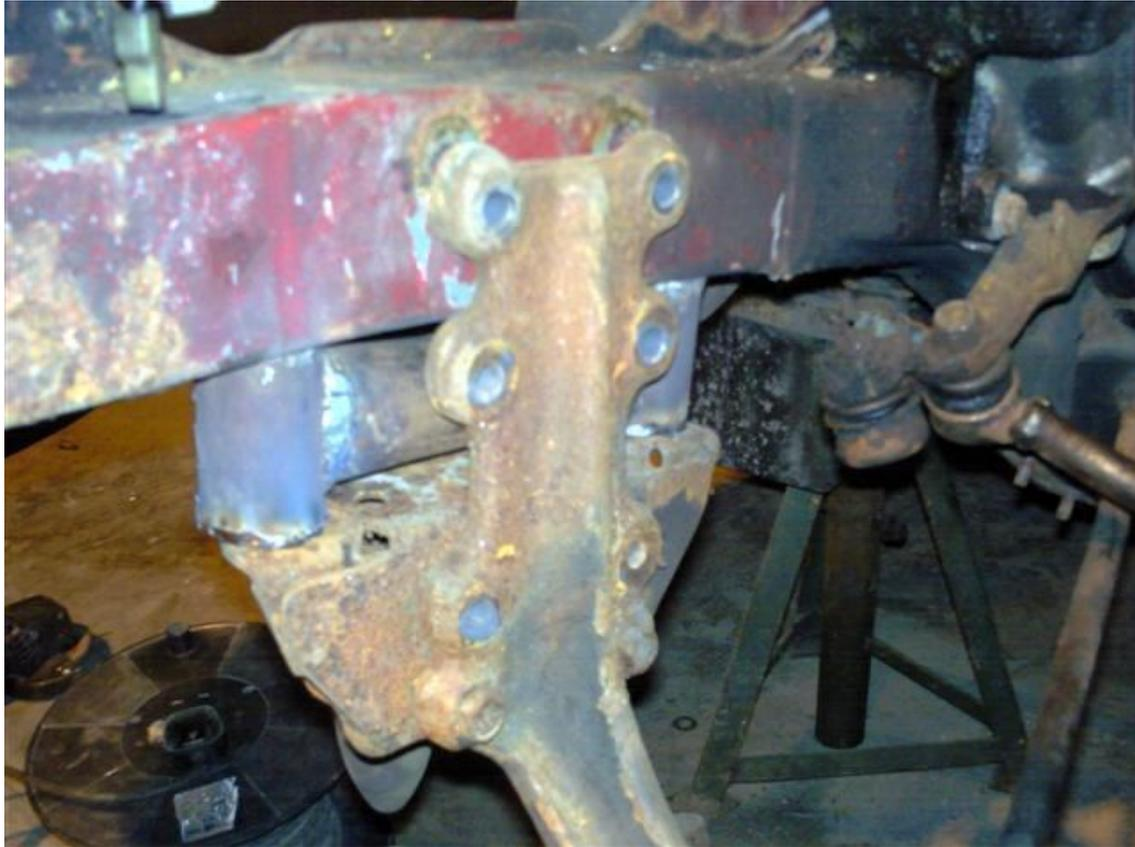
now you need your donor cross member. you need to cut underneath the 3rd bolthole down. This is so that you have enough holes for the engine mount etc etc to stay in the standard place when the whole thing is finnished. should look like this:
