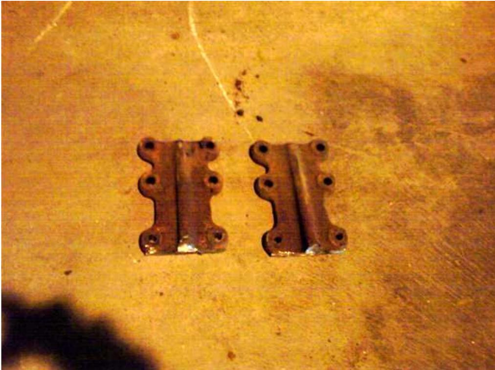
you can see that these are the top bits of the donor cross member. You need to clean the edge up that you have cut, and make sure you have a good chamfer ground all the way around it, so that the weld can get a good penetration later.
