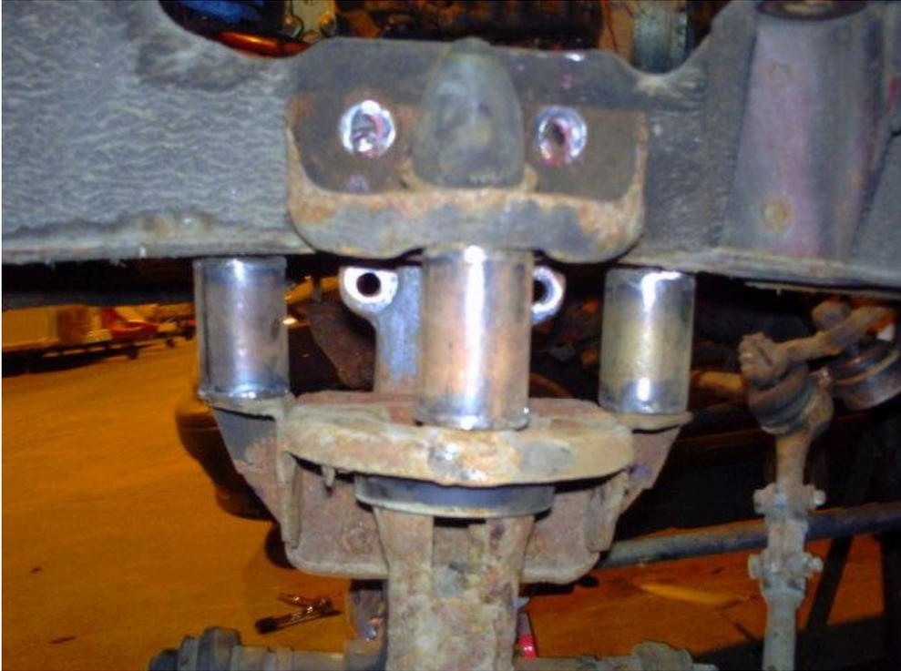
I then made braces to go in between all of these, to give the whole thing a lot of strength. I didn't take a photo if the in between, but I used the same spec tube as I did to make the spacers, and ended up with this:
