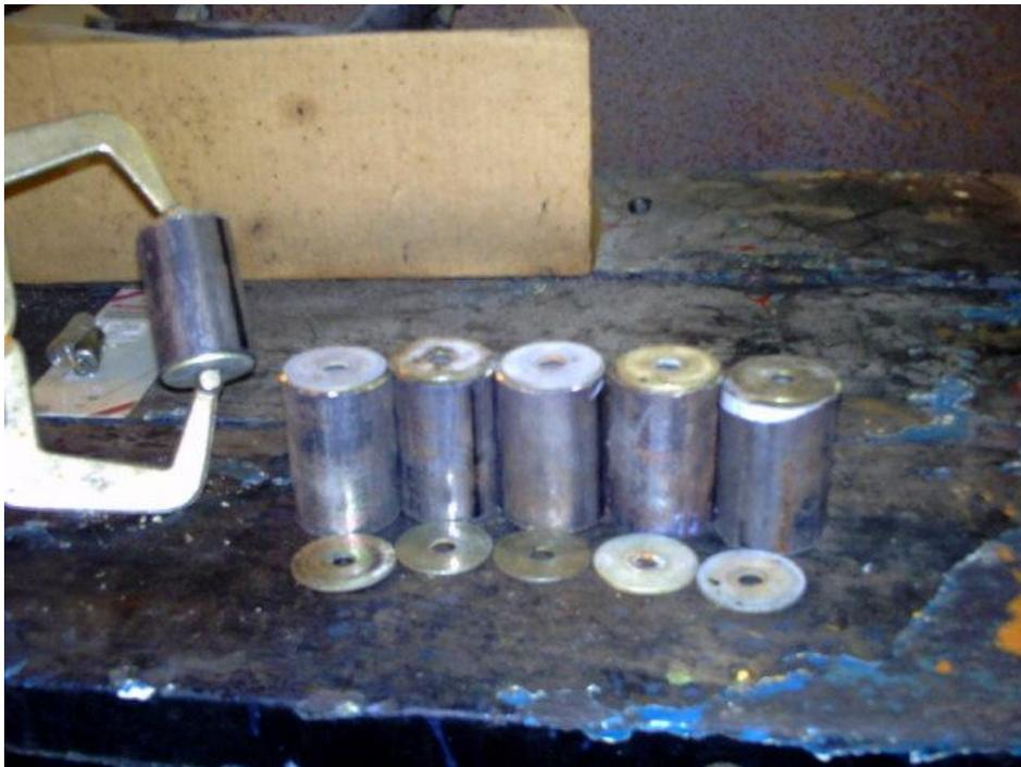
Weld one washer to one end of each tube. leave the other one off, as the bolts that come through the chassis to mount the cross member are captive, and REAL hard to get out without making a mess.
