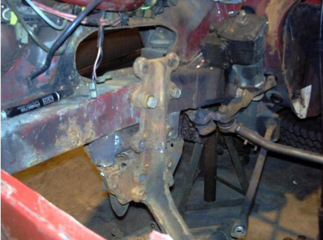
As you can see, the bolt holes for the top wishbone are in the standard location, as are those for the engine mounts. Nice eh 😊😊
